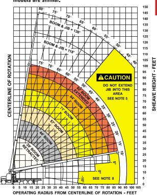
Area of Operation DO NOT OPERATE IN THIS AREA WITHOUT FRONT STABILIZER DEPLOYED
